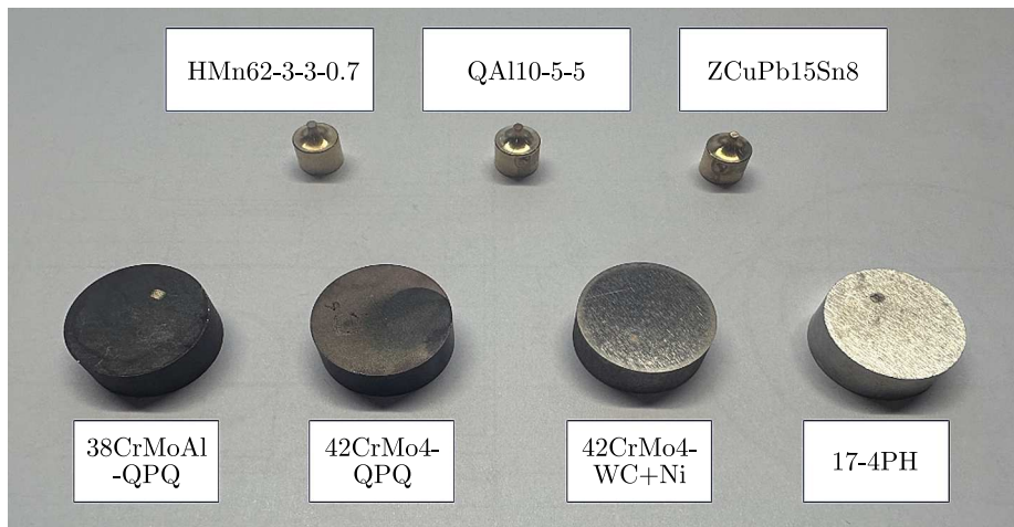
Fig. 2. Representation of slipper/eccentric cam pin-on-disc tribopairs
