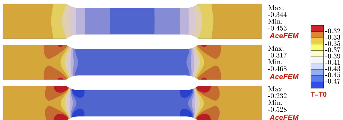
Fig. 4. Temperature distribution for slow, medium rate and fast processes (top, middle and bottom, respectively) at the end of simulation
