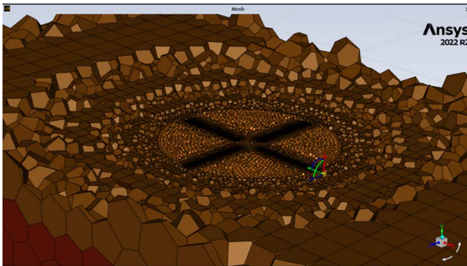
Fig. 6. Polyhexcore mesh of fluid volume elements
