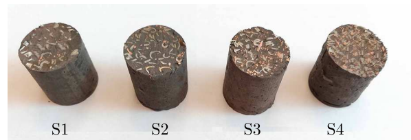
Fig. 3. Samples tested in compression test
