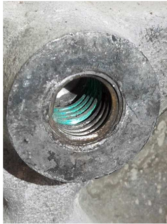
Fig. 2. Support hole thread the gearbox case
