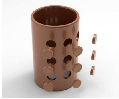
Fig. 2. Representation of L161 disc specimens made from the complete liner
