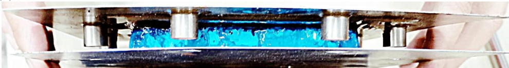
(c) Two layers (10 mm + 5 mm) diameter ceramic ball protective structure
